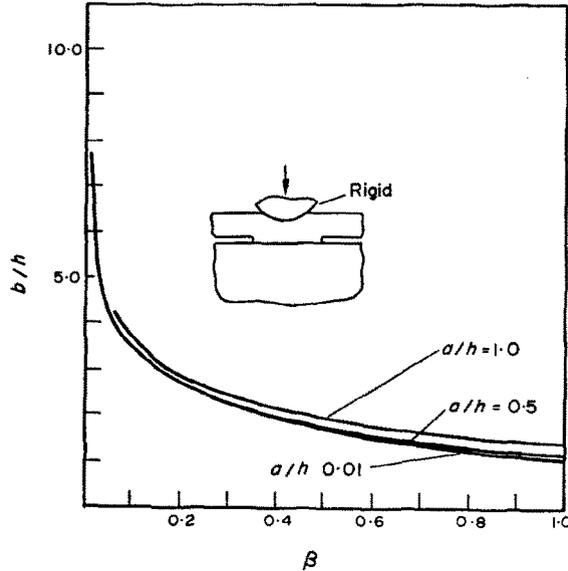
Fig. 8. Layer-half space contact radius  $b$  for loading by a rigid spherical stamp.
