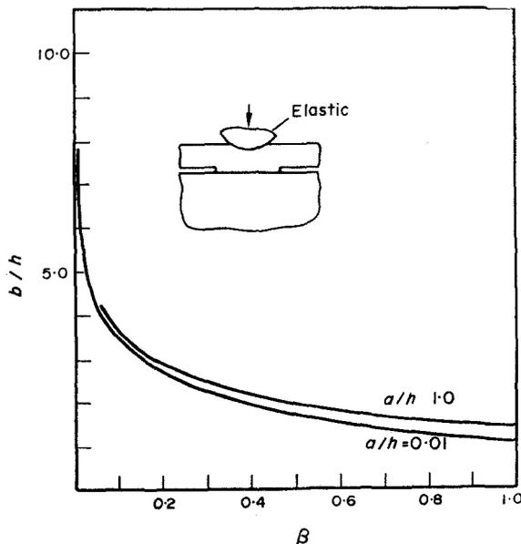
Fig. 14. Layer-half space contact radius  $b$  for loading by an elastic stamp.
