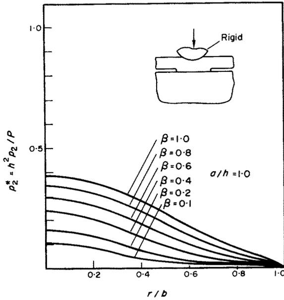
Fig. 12. Contact pressure between the layer and the half space for  $a/h = 1.0$  and for loading by a rigid sphere.
