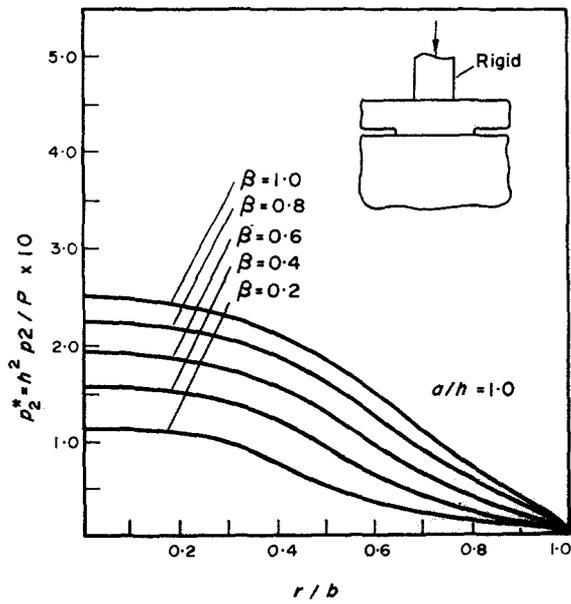
Fig. 5. Contact pressure between the layer and the half space for  $a/h = 1.0$  and for loading by a flat stamp.
