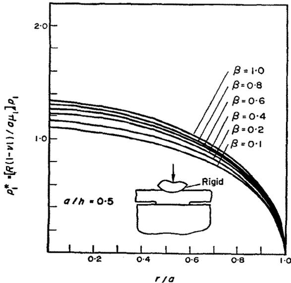
Fig. 9. Contact pressure between the rigid spherical stamp and the layer for  $a/h = 0.5$ .
