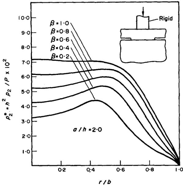
Fig. 6. Contact pressure between the layer and the half space for  $a/h = 2.0$  and for loading by a flat stamp.
