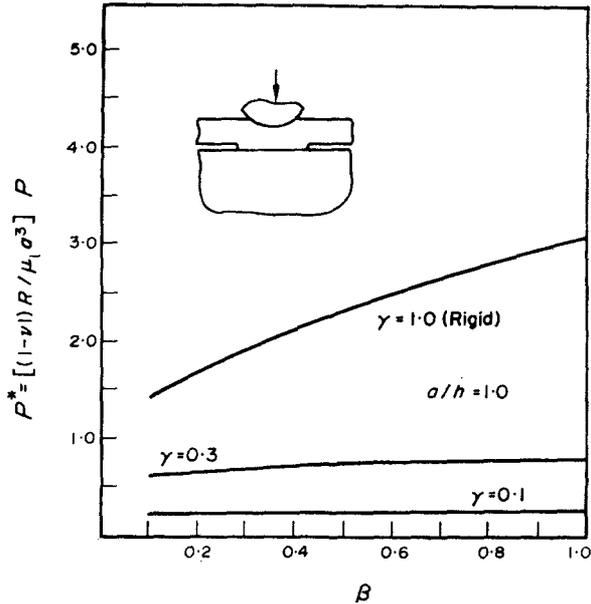
Fig. 17. Total transmitted force  $P$  vs the layer-subspace material constant  $\beta$  for various values of stamp-layer material constant  $\gamma$ , and for  $a/h = 1.0$  in loading through an elastic sphere.
