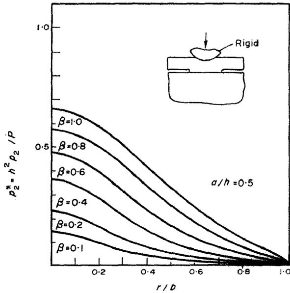
Fig. 11. Contact pressure between the layer and the half space for  $a/h = 0.5$  and for loading by a rigid sphere.
