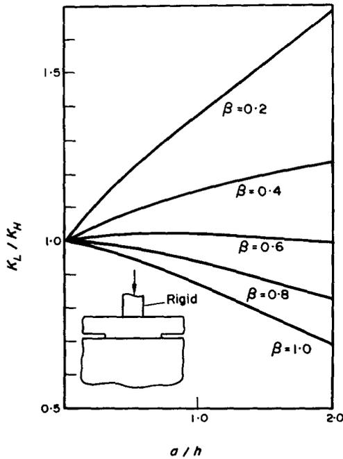
Fig. 7. The stress intensity factor ratio for the flat-ended rigid stamp.
