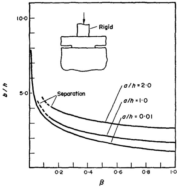
Fig. 2. Layer-half space contact radius  $b$  for loading by a flat-ended rigid stamp of diameter  $2a$ .
