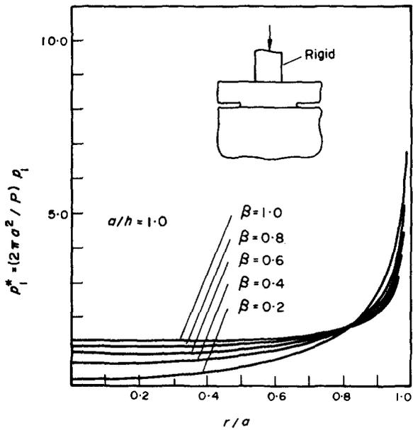
Fig. 3. Contact pressure between the flat stamp and the layer for  $a/h = 1.0$  and for various layer-half space material combinations  $\beta$ .
