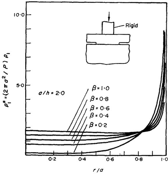
Fig. 4. Contact pressure between the flat stamp and the layer for  $a/h = 2.0$ .
