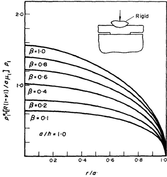
Fig. 10. Contact pressure between the rigid spherical stamp and the layer for  $a/h = 1.0$ .
