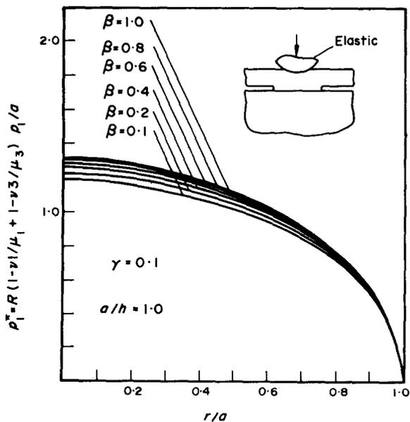
Fig. 16. Contact pressure between the spherical elastic stamp and the layer for  $a/h = 1.0$  and  $\gamma = 0.1$ .
