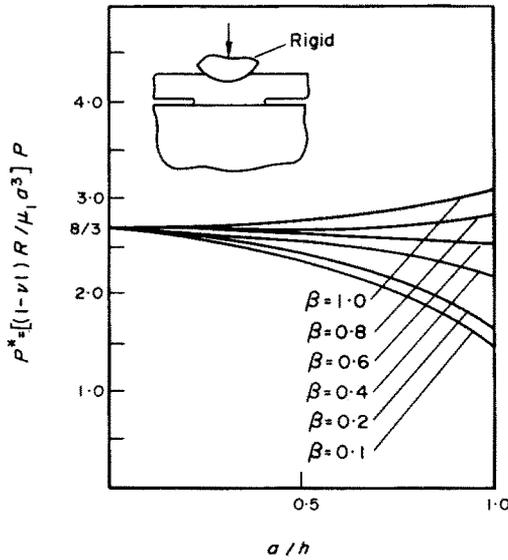
Fig. 13. Total transmitted force  $P$  vs the stamp-layer contact radius  $a$  for various layer-half space material combinations  $\beta$  and for loading by a rigid spherical stamp.
