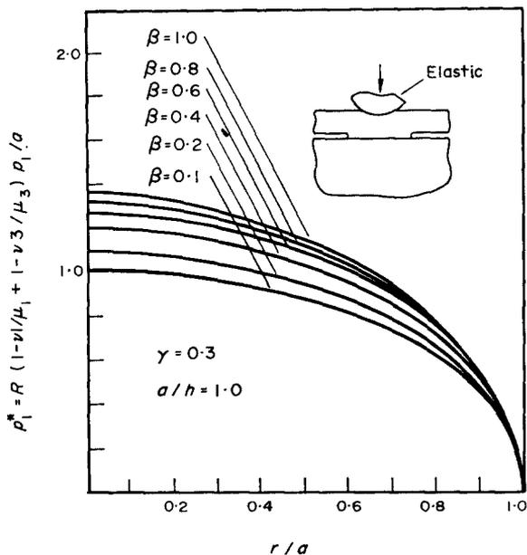
Fig. 15. Contact pressure between the spherical elastic stamp and the layer for  $a/h = 1.0$  and  $\gamma = 0.3$ .
